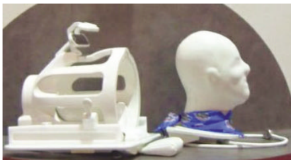
Figure 3 A whole brain transceive coil and head phantom offered within a commercial package. The package includes paradigm presentation, communication gear, and head stabilizing attachments. The coil is curved toward the superior portion of the head for increased sensitivity in that region. Picture courtesy of MRI Devices Corp. (Table 1, vendor 14). [Color figure can be viewed in the online issue, which is available at www.interscience.wiley.com .]
