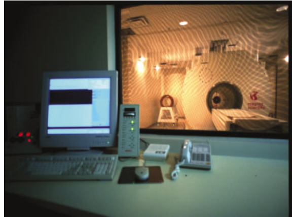
Figure 1 The 7-T 900-mm clear bore fMRI magnet used for human research at the University of Minnesota. The view is from the operator console through a screened window into the iron- and RF-shielded magnet room. A patient bed and a whole-body shim and gradient coil assembly is installed in the magnet. An insertable head gradient set can be seen on a cart outside the magnet. The operating room contains all controls for executing MR experiments, paradigm presentation, and patient communication. Picture courtesy of Prof. Kâmil Uğurbil, University of Minnesota. [Color figure can be viewed in the online issue, which is available at www.interscience.wiley.com .]
