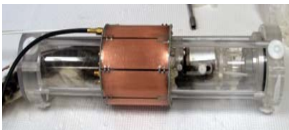
Figure 1. Commercially available restraint apparatus for high resolution fMRI of conscious animals.
